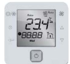
The thermostat must be fixed at a height of 1,5 metres from the ground and all possible interferences must be avoided: sun, outdoor air, internal heat sources... Mount the thermostat to the wall using the bracket, do not leave it hanging from the wire or embedding it in the wall.
